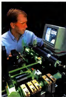
Beams of light are used to record a holographic image into the storage medium
